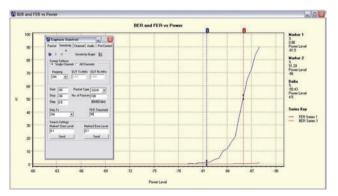
Automatic sensitivity search measurements display the FER/BER performance of an EUT with decreasing power into the receiver. Tests can be performed on all supported standard rates and EDR packet types.
