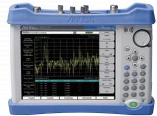
The MT8212E/13E incorporates a spectrum analyzer and cable/antenna analyzer as the basic configuration with options supporting 3G, LTE, and WiMax modulation analyses. In addition, it has all-in-one support for measurements such as cable and antenna VSWR, Distance To Fault (DTF) etc. The easy-to-use touch panel with screen modes for various lighting environments helps improve work efficiency.
