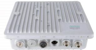
The MS27102A is a water and corrosion-proof cabinet enables spectrum monitoring at outside locations. It can be remotely controlled over Ethernet from the back office for on-site radio-wave monitoring. Dedicated software supports long-term recording as well as estimates of inspection target signal source locations using multiple device data.
