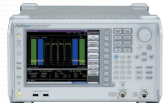
Signal Analyzer MS2690A/91A/92A has the excellent total level accuracy, dynamic range and performance of a high-end spectrum analyzer. Not only can it capture wideband signals but FFT technology supports multifunction signal analyses in both the time and frequency domains. Moreover, the built-in signal generator function outputs both continuous wave (CW) and modulated signals for use as a reference signal source.
