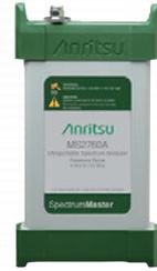
The MS2760A is the world's first handheld millimeterwave (mmWave) spectrum analyzer to provide continuous coverage from 9 kHz up to 110 GHz. It is ideal for the growing 5G network development market, as well as other fast growing mmWave applications, like IEEE 802.11ad/WiGig, E-band microwave wireless communications, satellite communications, and automotive radar.
