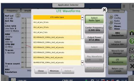
Select Radio type to send the correct commands to initiate a LTE waveform transmission.
