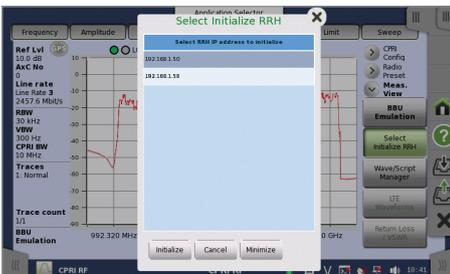
Select RRH to test, IP address of the RRH shows up in order of discovery.
