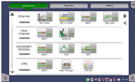
The MT1000A displays all the applications available from the installed modules. For CPRI RF measurements, select the CPRI RF application icon.
