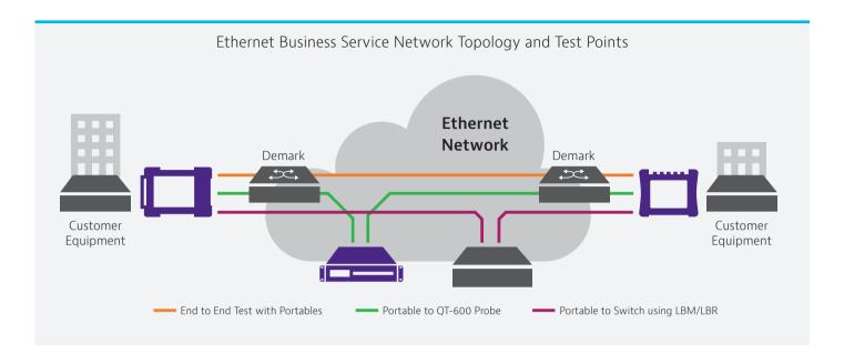
The diagram above shows the "local" TBERD represented on the left side and the "remote" TBERD on the right. The most common service activation use case is a loop-back of the remote device and in this case, the device will be the remote TBERD.
