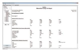
Making Bluetooth low energy measurements on a device with an HCI interface can be fully automated from the [Script Testing] tab. The user simply selects and configures the required test cases and clicks to execute the script. The test results display in a report that can be printed or saved by the user.
