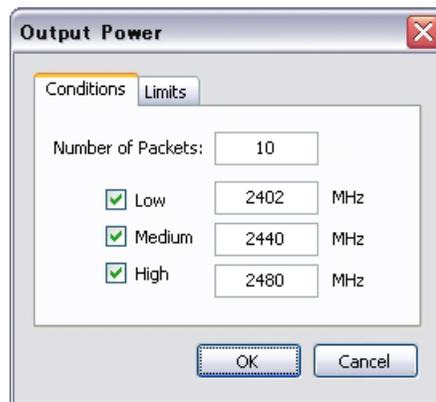
**Figure 6-5.** Output Power Test Conditions and Limits
