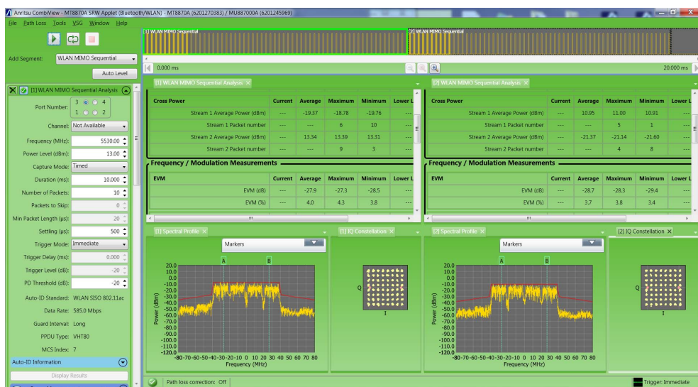
Figure 6-6. Sequential MIMO 2 x 2 Measurement
