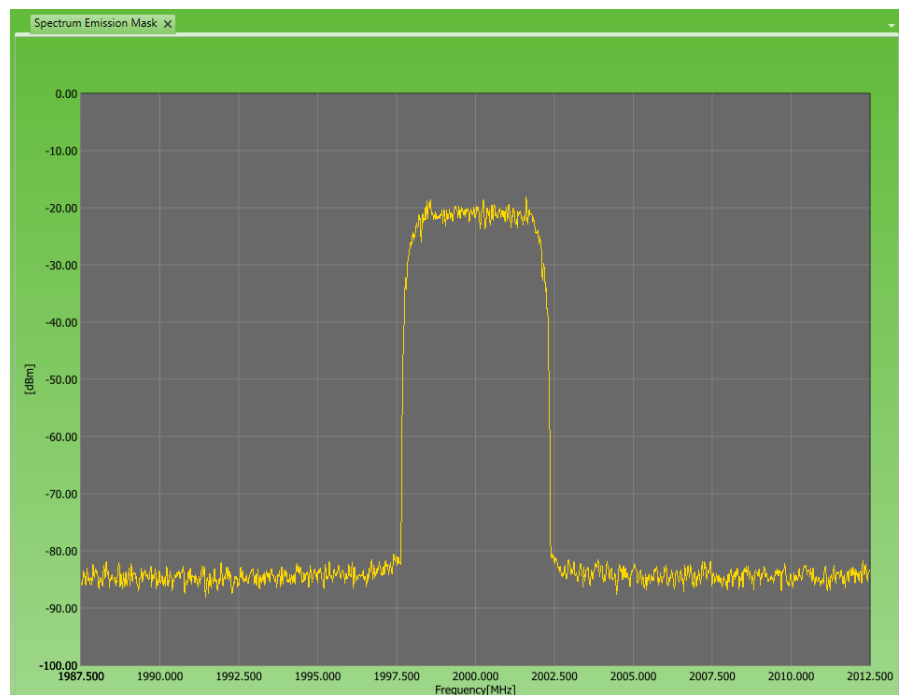
Figure 3.2.2-1 W-CDMA (Spectrum Emission Mask) Graph
