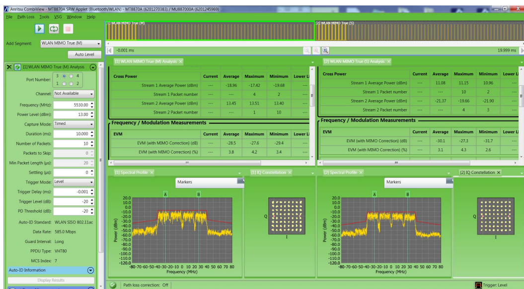
Figure 5-5. True MIMO 2 x 2 Measurement
