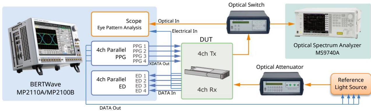
Fig. 2 BERTWave Measurement System (using MP2100B/MP2110A with Opt-014 and Opt-023 installed)
