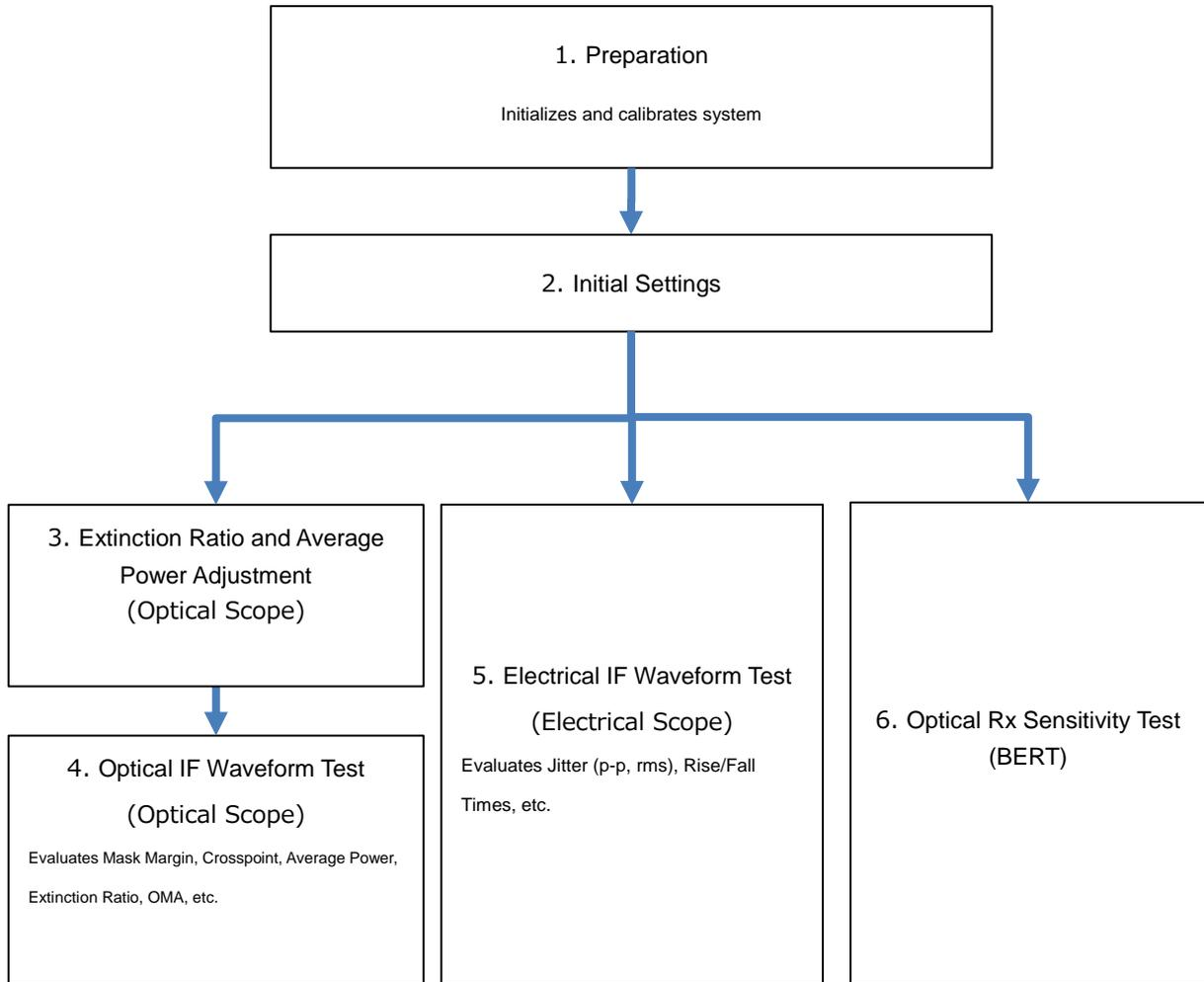
Fig. 3 Overall Sequence of Optical Module Evaluation
