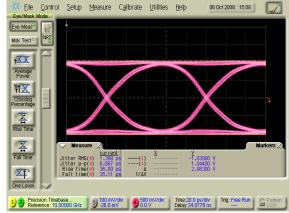
Figure 4.14: MU181020A-011 Waveform with LPF
