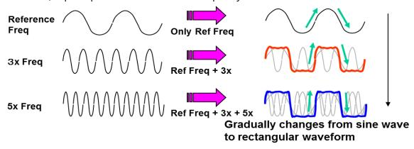
Figure 2.1: Compositions of Rectangular Waveforms
