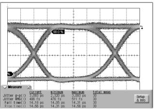
Figure 3.1.2: Waveform Measured with 70-GHz Scope
