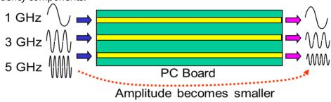
Figure 2.2: Transmission Path Loss
