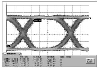
Figure 3.2.2: Waveform without Precision Trigger
