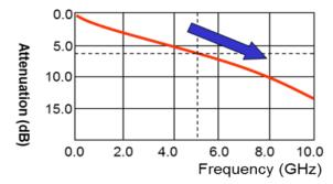
Figure 2.3: Frequencies and Attenuation
